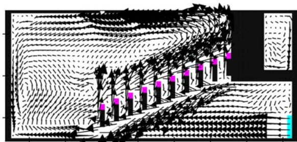
Fig. 13. Airflow pattern at section yz19. Air terminal devices at the back
